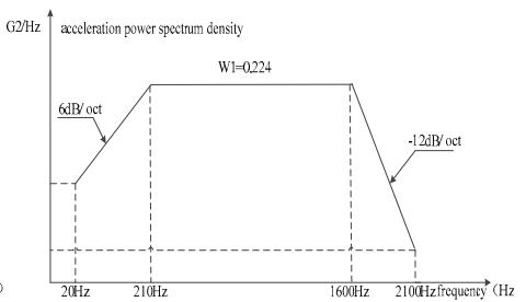
Fig. 3. Vibration spectrum
