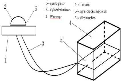
Fig. 1. Structure of sun sensor
