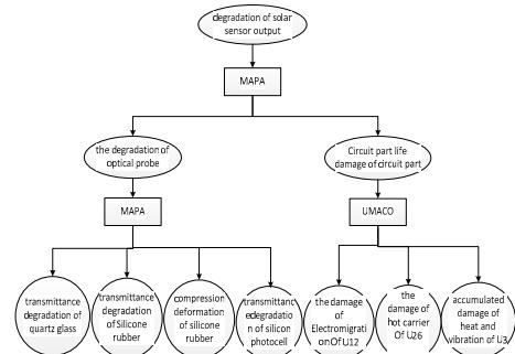
Fig. 6. The failure mechanism tree.
