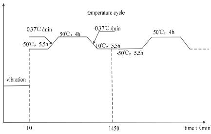
Fig. 2. Sun sensor's comprehensive stress profile of simulation analysis
